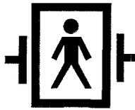
This equipment provides a degree of protection against electric shock to TYPE B as defined in IEC60601-1. This equipment has an F type applied part capable of withstanding the effects of defibrillator discharge
