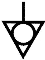
This symbol indicates the conductor that may be used to provide potential equalization between the equipment and the installation busbar.
